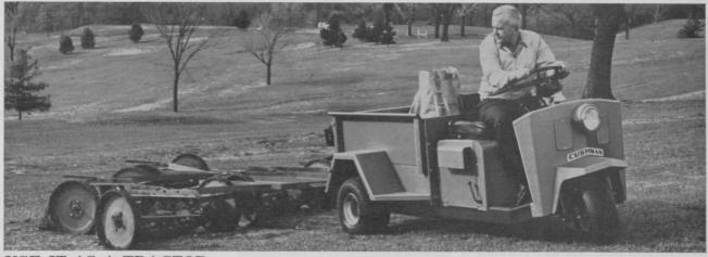
USE IT AS A TRACTOR to pull gang mowers or other non self-propelled equipment. Big 9.50 x 8 traction-tread tires give plenty of traction without
