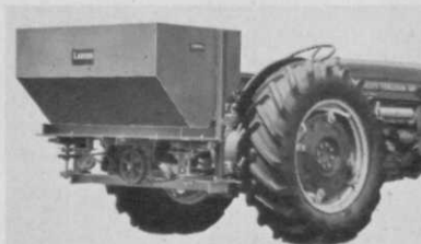
MODEL 413 "PIGGYBACK" —15 cu. ft. capacity. All the features of the 411 BROADCASTER. Attached to tractor by simple 3-point hook-up. Three-point hitch adapters available for all tractors.
