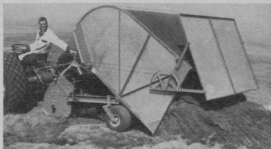
The operator easily empties the 5-cubic-yard hopper from the tractor seat.
