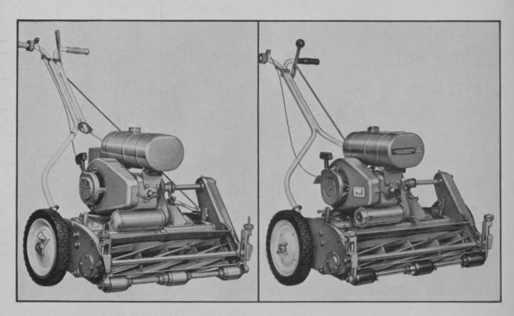
**New Jacobsen Greens Mower** with Space Age SSI (Solid State Ignition) completely eliminates cams and points. Fool proof integrated circuit provides a consistent, high intensity spark *indefinitely*. Heat and humidity never affect ignition. You get new dependability and longer engine life. SSI is warranted for 2 full years.
