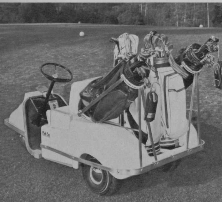
Above, Stevens "Four-Bagger" golf car made of fiberglass. An aluminum bracket was mounted on both the right and left rear fenders to the standard Club Car allowing easy access to golf clubs in both bags.
