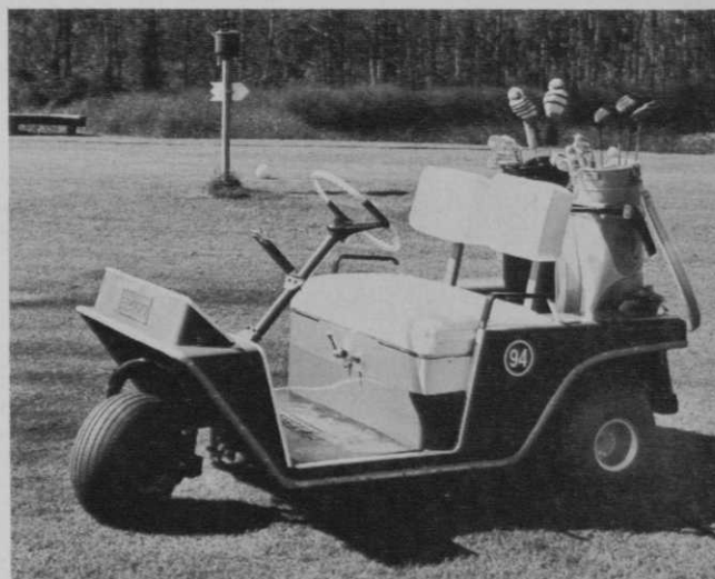
Above, E-Z-Go's model x-440 electric golf car, built with an all steel welded construction and all steel body with baked on automotive enamel. Model x-440 comes with tiller or wheel steering.
