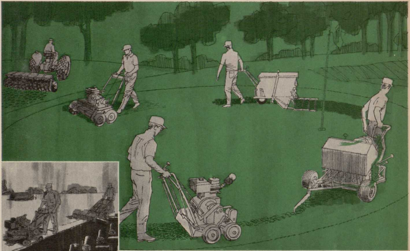
RYAN EQUIPMENT above (left to right): Tractor-drawn RENOVAIRE for aerating large areas; SPIKEAIRE power disc spiker; MATAWAY power rake or vertical mower; SPREAD-RITE top-dresser, fertilizer spreader; and GREENSAIRE coring aerator.
