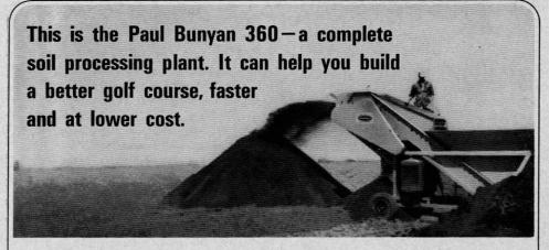
It can process up to 100 cu. yds. of soil mix in an hour. Raw materials in one end—clean, easy-to-work amended soil mixes out the other (mixes that speed grading and seeding). It features a patented high-speed cleated-belt mechanism that delivers a 5-step soil preparation that is continuous and thorough.
