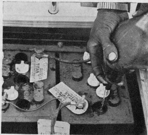
Extreme care is given each battery to ensure proper fluid level and good connections.
