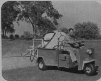
Boom spraying on a green with the popular Turf-Truckster cuts spraying time to minutes; also operates as boomless sprayer.
