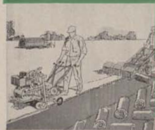
RYAN SOD CUTTER followed by world's first mechanized sod rolling machine.
