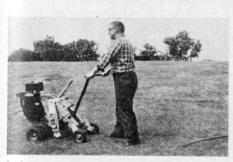
**Sod-Master** has come out with the Pipe Piper, a trencher which lays wire, cable and pipe underground without removing turf.
