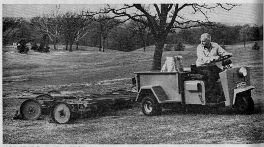
**USE IT AS A TRACTOR** to pull gang mowers or other non self-propelled equipment. Big 9.50x8 traction-tread tires give plenty of traction without damaging turf. Six speeds for-
