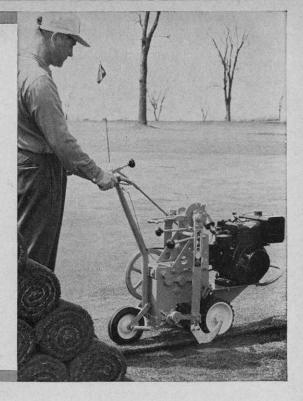
This versatile, self-propelled unit will cut 100 sq. ft. of sod per minute (over 11 sq. yards) so that you can completely strip old sod from a tee or green in minutes, then cut new sod in your sod nursery just as fast for a complete replacement job in less than a day's time! By ordering
