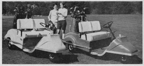
Pioneering in fiberglass bodies and development of the only aluminum frame used in golf car manufacturing enables us to market a 2-passenger golf car that weighs only 350 lbs. plus 360 lbs. of batteries for an operating weight of 710 lbs. This is 200 to 500 lbs. lighter than other golf cars and results in far less wear and tear on fairways, turf and golf car batteries.
