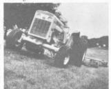
A differential lock feeds power to both rear wheels regardless of traction. No spin-out. No gouging of turf even when you start up from a dead stop on a slope. On side hills it holds the nose straight and prevents downdrifting.
