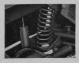
New rear suspension combines coil springs, hydraulic damper and torsional stabilizer — provides absolute maximum stability and comfort.
