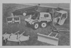
The new 18 hp. Bolens GK is equipped for year round use. Attachments for frame-steering vehicle include: 72-inch 4 blade rotary mower with retractable wing sections; 48-inch snow caster; transport trailer; 1-cu. yd. utility dump cart with removable tail gate section; all-weather cab with tempered glass, removable doors, wind-shield wiper, emergency light; and 54-inch heavy-duty snow/grader blade with hydraulic angling.
