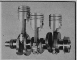
block. Chrome-faced rings. Top rings in hard, heat-resistant ring groove inserts. Bigger combustion chambers. Great new engines-thrifty, smooth, and tough-for great new tractors.
