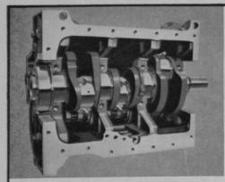
Three-cylinder design puts bigger, stronger moving parts in a shorter, more rigid engine. Huge crankpins solidly supported between 3%-inch diameter mains. Bearing area unequalled in this power class. Rigid cylinder
