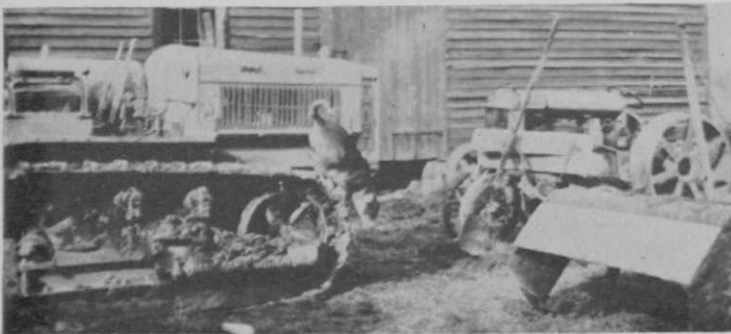
Equipment looked like this 40 years ago. Cat 30 is at left, Fresno scraper at right, Fordson is in background.
