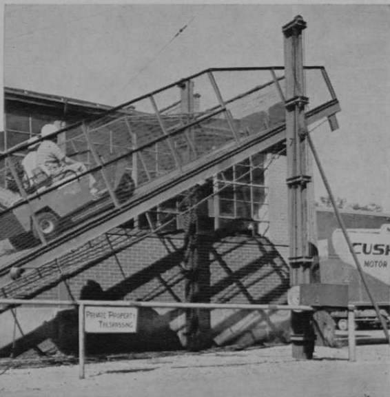
This is how the hill testing unit, which is higher than adjoining one-story building, looks from the side. (Inset) Test drivers always wore crash helmets while they were putting prototype models through paces in and out of ditches and over the roughest kind of terrain.
