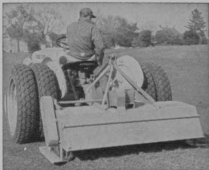
"The MASTER VERTI-GROOVE with rotating renovating blades and stationary slicing knives; used in combination for thorough renovation, separately to slice or spike."
