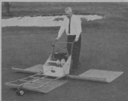
The POWER DRAG mats 9½' swath. Easy to transport — folds for storage.
