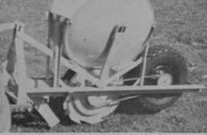
Revolving discs keep sprigs in place for automatic feeding. One man operation.
