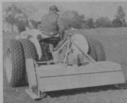
The MASTER VERTI-GROOVE designed with Renovating Reel and Slicing Blades; used in combination for thorough renovation, or separately to slice or spike.
