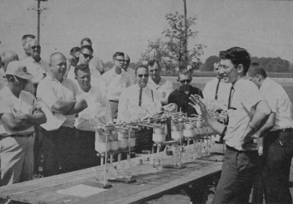
Soil infiltration rates are explained to fieldday visitors by Paul Rieke, MSU soil scientist. He poured water into different soil mixes to show the rate of movement through them. This basic experiment is helpful in the selection of soils for putting green mixtures.
