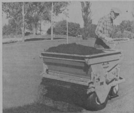
◀ **See how Ryan units team up to do more jobs:** To get maximum results from aerating, follow it up with uniformly distributed applications of top dressing, turf builder or fertilizer. The big capacity self-propelled Ryan Spread-Rite handles all these materials . . . exclusive "live action" hopper feeds them evenly, damp or dry, over a full 39" swath. See your Ryan distributor or write:
