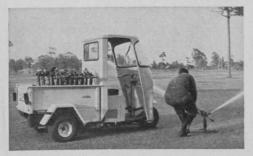
NIGHT WATERING. Load the sprinkler heads into your big Cushman Truckster and start out. Big 9.50 x 8 tires allow Truckster to drive freely, even on wet fairways.
