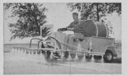
**SPRAYING.** Built especially for spraying greens, this boom sprayer covers 16-foot wide strip thoroughly and evenly, is operated by Truckster engine through power take-off. Boom and spray rig can be removed in minutes.
