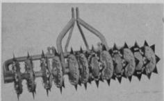
swath and are designed for use with tractors that have a 3-point hydraulic hitch. Each operating wheel is mounted with a set of eight aerating tines. The Tracaire, with a complete set of coring, slicing and renovating tines, can be used throughout the turf growing season for a complete building and improvement program, according to Ryan.
