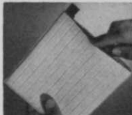
Close-up of single positive plate in protective polyethylene jacket
