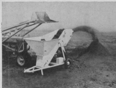
BUILD — Royer soil shredder-blender
