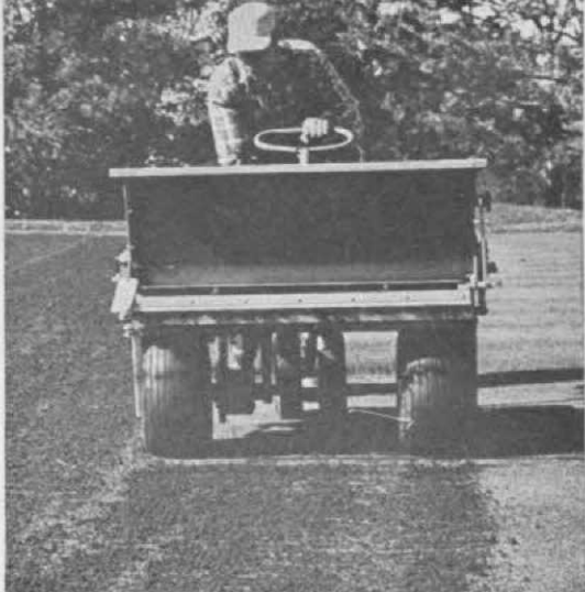
Spreading is uniform over full width of the spreader—so non-marking wheels do not run on fresh top dressing.
