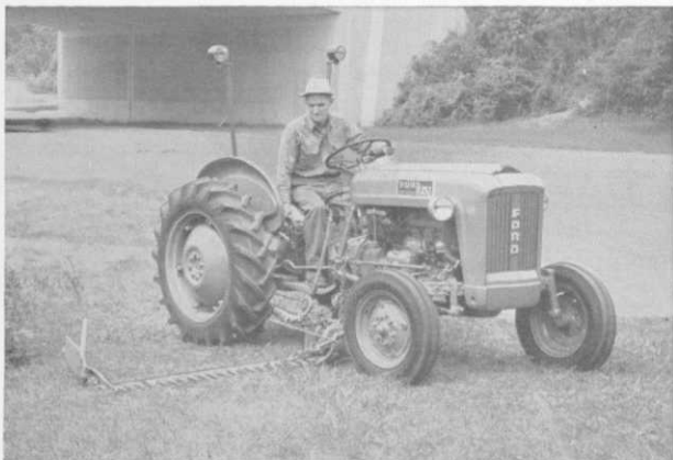
For all cutter bar mowing, Ford mowers are available in 5, 6, and 7 foot cutting widths. Curb lift provides up to 10½ inches of clearance under the inner shoe (except with LCG tractors).
