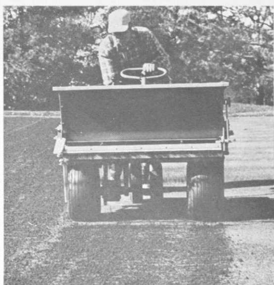
Spreading is uniform over full width of the spreader—so non-marking wheels do not run on fresh top dressing.
