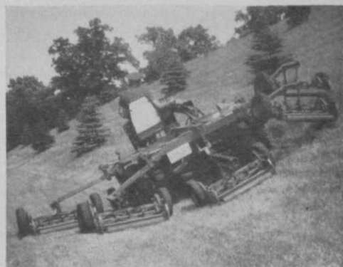
If man can stay in the seat, Parkmaster will hang on the hill and mow fast. Outboard gangs on uphill side add traction.
