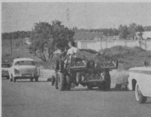
Go from job to job up to 40 m.p.h. Parkmaster's rugged Spartan gang mowers tuck up for 8-foot transport width.
