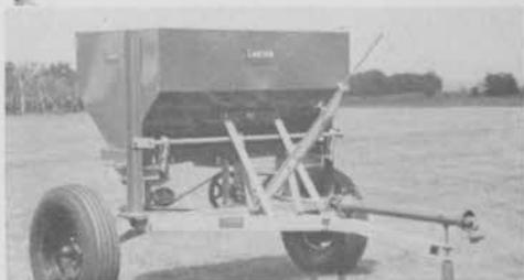
In the new line is the 410 trailer type broad-caster, with 15 cu. ft. hopper, said to be ideal for courses. A modification of the 410 is the 403 "Piggyback" with 15. cu. ft. capacity and 3-point tractor hookup. All Larson models cast spreads up to 50 ft. in width. Complete information on the line can be obtained from L. L. Larson Machine, Inc., Princeville, Ill.
