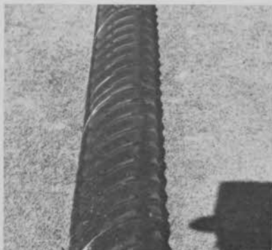
Section of Orangeburg type tile showing holes for water entrance.
