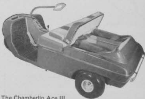
The Chamberlin Ace III, manufactured by Chamberlin Metal Products Co. Frankfort, Michigan. Powered by Kohler 7 HP Engine K161S.
