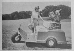
Golfkar, it is powered by a 7 hp engine (Kohler K-161S) and is said to go 36 holes on two gals. of gas. An automotive type muffler combined with the fiberglass body restricts noise. The vehicle rides on aircraft type balloon tires, weighs about 450 lbs. and has a 53-in. wheelbase. It is equipped with foam cushion seats, rubber cushion mounting on the front wheels and has an automotive type coil suspension of the rear wheels.
