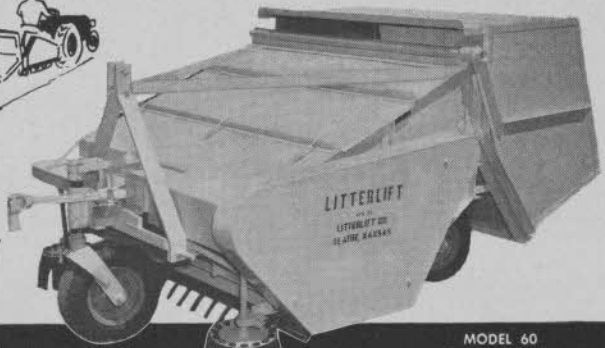
MODEL 60 Tractor mounted unit with self dumping hopper
