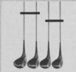
"Ordinary" sets are only half-matched. Diagram shows how identical shafts are used for more than one club head. Although head weights vary, shaft action does not. No more than half the clubs in "ordinary" sets are truly matched in balance and "feel."
