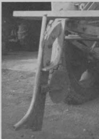
The Haines root pruner as modified for laying underground cable.
