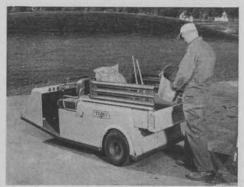
tank with electric indicator and outside fill. Other engine features include an extra heavy crankshaft, 3-qt. oil capacity, stellite exhaust valves and seats, twin power magneto ignition, etc. The tiller bar is said to be vibration free. Top speed of the Workmaster is between 7 and 10 mph. Tires are of the low-pressure type and the front end spring suspension makes for easy riding.
