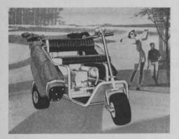
ered vehicle that weighs about 200 lbs. The 4 hp engine has an extra low-tone, high volume muffler and has either an easy-spin recoil or electric starter. Accelerator and brake are located on a single pedal and the low profile pneumatic tires have extra wide rims for easy riding. The Par-Pony can be loaded into a station wagon by one person although there is a
