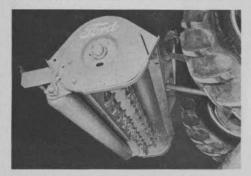
plement Div. represents a new concept in mowers, according to the manufacturer. In contrast to the scissors action of the sickle bar, to the reel-type whose blades cut against a stationary bar, and to the rotary whose blades move in a horizontal plane, the flail mower has free swinging blades which hang from a rotor parallel to the ground. It is said that this construction virtually eleminates the hazard of objects being thrown beyond the protective shield of the unit.
