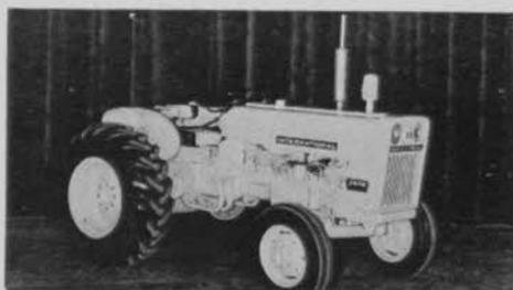
Designed especially for use in landscaping, leveling, mowing, and a wide variety of applications is the International 2404, equipped with a 4-cylinder engine with a rated 47 bare engine horsepower.
