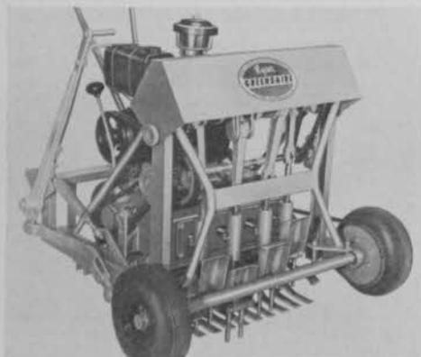
so it can cover a maximum of 6,000 sq. ft. an hour. The precision-built turf aerator is said to remove 30,000 clean-cut, evenly spaced cores in every 1,000 sq. ft. of turf, thus creating as many reservoirs that bring air, mois-
