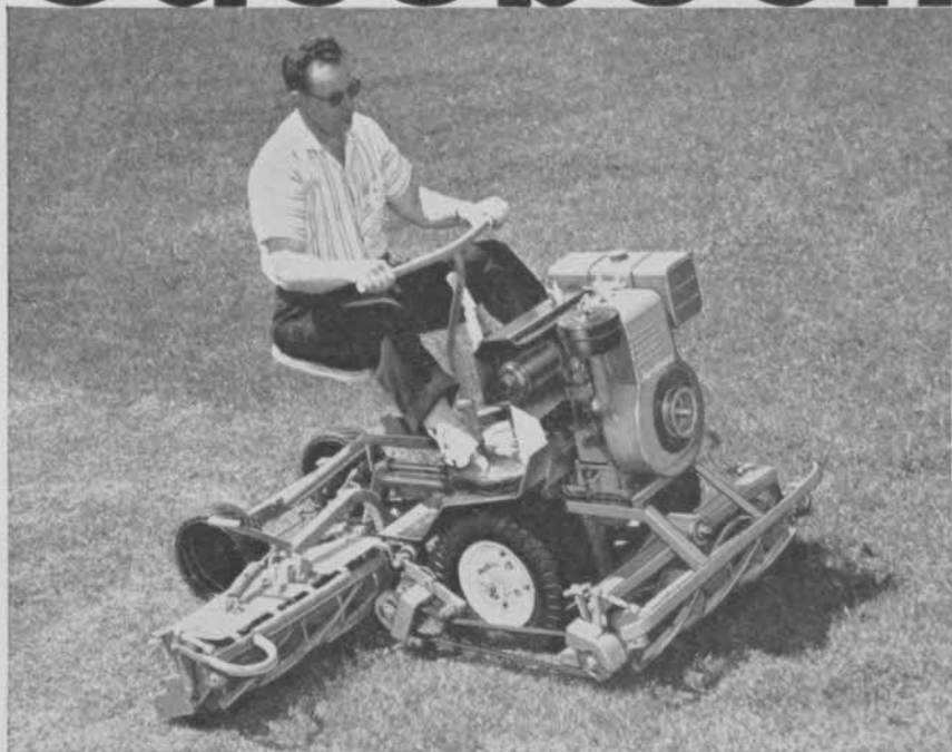
Turf-King 76—Three articulated power reels operate ahead of all wheels. Retractable wings cut at 30° angle, up or down.
