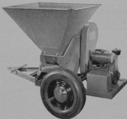
Royer Shredder Model 16, with Batch Hopper. Capacity up to 20 cu. yds./hr.
