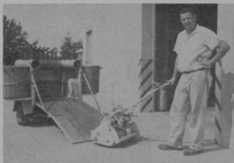
Bob Grant stands alongside converted maintenance vehicle. Sprinklers are carried inside pipe and baskets on side are for green clippings.
