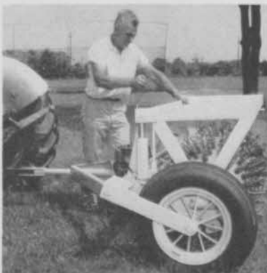
Hydraulic control provides fast lowering and raising of Spoons.
