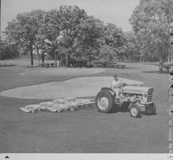
**Stamina on a budget!**... Year-in and yearout dependability combines with rock-bottom operating cost in the 40-hp\* International 240—ample power to pull a 7-gang mower. When you need extra "oomph," look at the 47-hp\* International 340, available with 10speed Torque Amplifier Drive. Handles up to nine gangs... up to 1,600 lb with loader.
