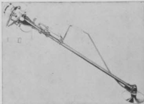
models. Called the Brushking and known as Model 660, the unit provides 3 hp. The added power is said to virtually eliminate any tendency of the blade to bind even when cutting through dense brush or trees up to 9-ins. dia. Vibration also is said to be effectively minimized.
