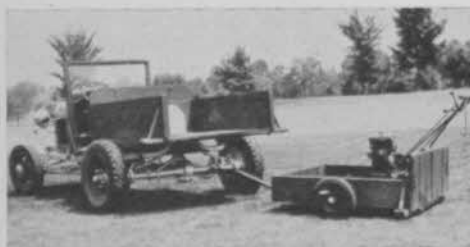
Brynwood loaded mower transport trailer with end gate in closed position. Note snap type closing fixture.
