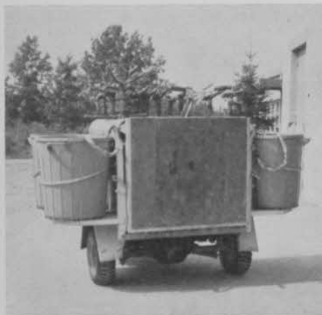
Loaded mower in Cushman pick-up. Four baskets are for grass clippings. Sprinklers are placed in circular openings in section of large size plastic pipe.
